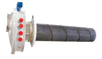
The HELIMAX™ is a next generation heat exchanger with Continuous Helical Flow Technology™ that enables ultra-high heat transfer unlike large, traditional heat exchangers with dead zones. Fluctuations within the heat exchanger to either the sheath temperature or the localized flow rate are common causes of coking, which can lead to system failures and expensive downtime.
