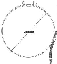
The stainless steel clamp allows temperature measurement without drilling or tapping which is ideal for measuring pipe temperatures.
