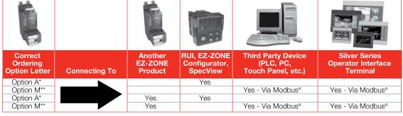
\*A = Standard bus used to connect to Watlow PC software, RUI, other EZ-ZONEs
