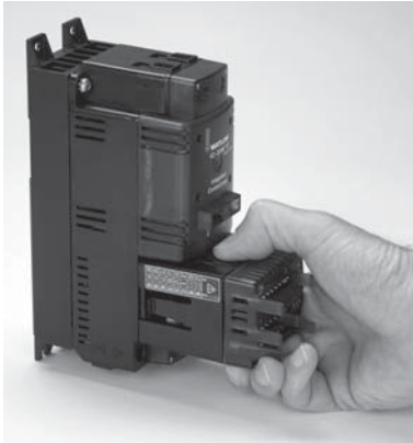
1. Pinch the release levers on the top and bottom of the control module and lift the right edge forward to detach the unit.
