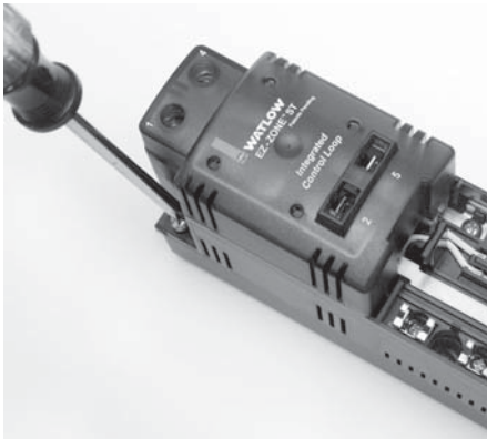
3. With a Phillips screwdriver, remove the two screws at the top corners of the controller.
