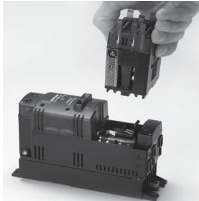
1. Pinch the release levers on the top and bottom of the control module and lift the right edge forward to detach the unit.
